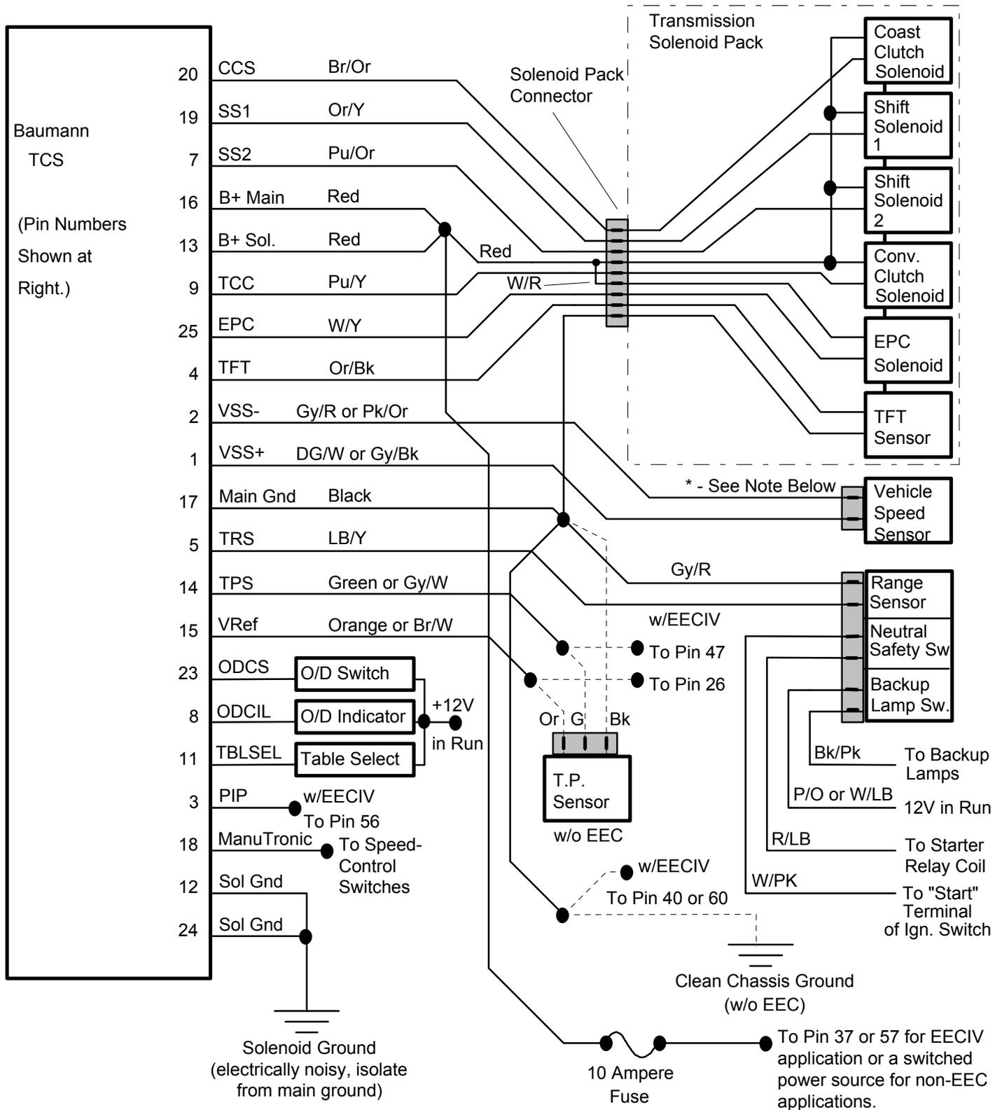
**Figure 3. Connection Diagram for E4OD Transmission**
